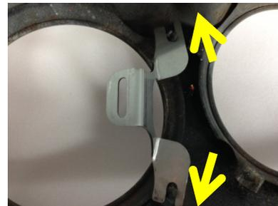
Bent MTBRGMK Installed in Dash
