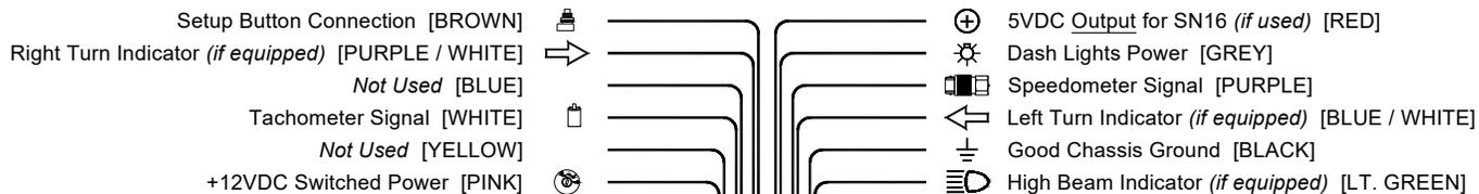
Turn & High Beam indicator leads are only used if gauge was ordered with indicator lights built-in.
