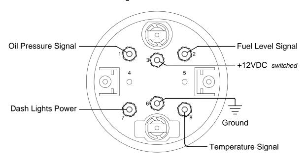
Older 3-3/8" quad gauges have alternate labeling as follows: 3 = B+, 6 = GND, 8 = 3, 7 = 4
