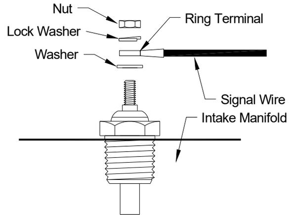
**Notice:** Avoid installing the temperature sender into the head of a late-model GMC engine. Even though the stock GMC sender may have been installed there, this opening is too close to the exhaust header and will most likely cause an improper reading.
