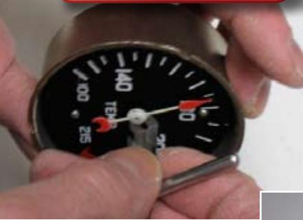
*This can be challenging, reusing the original pointer. Often they have to be "re-hubbed" to fit the shaft of a new instrument.*
