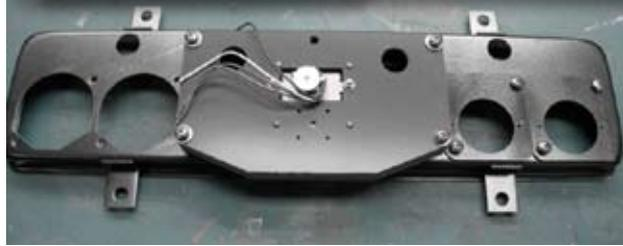
*Seen here from the back, the stock instrument cluster housing has been fitted in the middle with an adapter plate for the speedometer. The holes on the right have adapters for the new fuel and oil*
