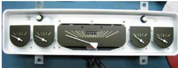
*New instrument faces were laser cut and printed to duplicate the originals.*
