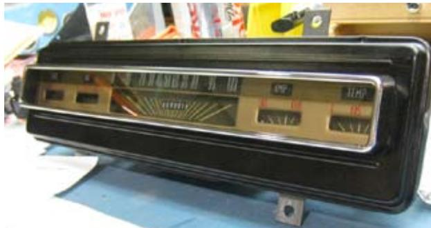
*Looking better than new, the refurbished instrument panel has up-to-date gauges and an easily programmable electronic speedometer.*
