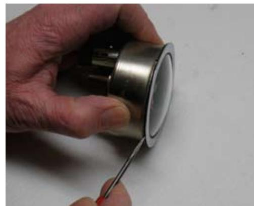
*Disassembly of the temp gauge began by carefully removing the rim from the housing.*
