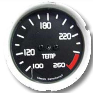
*Prior to reassembly the inside of the housing was painted white to brighten the normally poor night lighting of early instruments. Other than the increased range, the new gauge face is identical to the original.*
