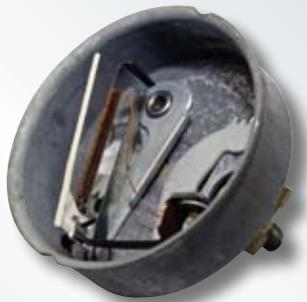
*Our vintage mechanical temperature used a Bourdon movement. The curved copper tube straightens when pressure is applied to it (due to oil pressure or expansion of the fluid in the tube).*
