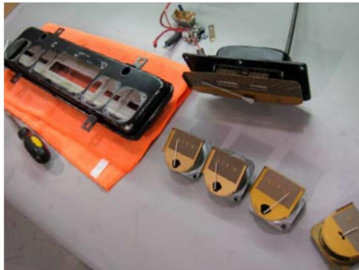
The gauges were removed from the panel, it was then bead blasted and the inside surfaces were painted white, adding reflectivity for improved nighttime lighting.
