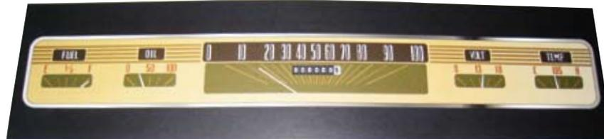
*A new face for the cluster was created, the oil pressure gauge now has a max of 100 psi rather than the original 50; note this version has a voltmeter and the finished product has what looks to be an ammeter.*
