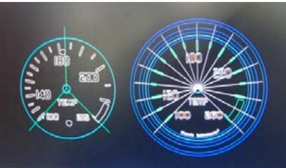
*The trick to installing a new movement in an old gauge is to match the sweep of the needle to the original. Originally the temp gauge read 100 to 215 degrees, with the same sweep it will now read 100 to 260 degrees.*
