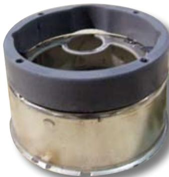
*To provide space for the updated internals a spacer was added to the back of the original housing.*
