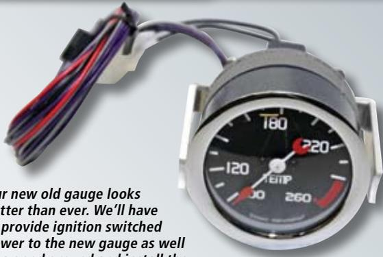
*Our new old gauge looks better than ever. We'll have to provide ignition switched power to the new gauge as well as a good ground and install the supplied sending unit.*
